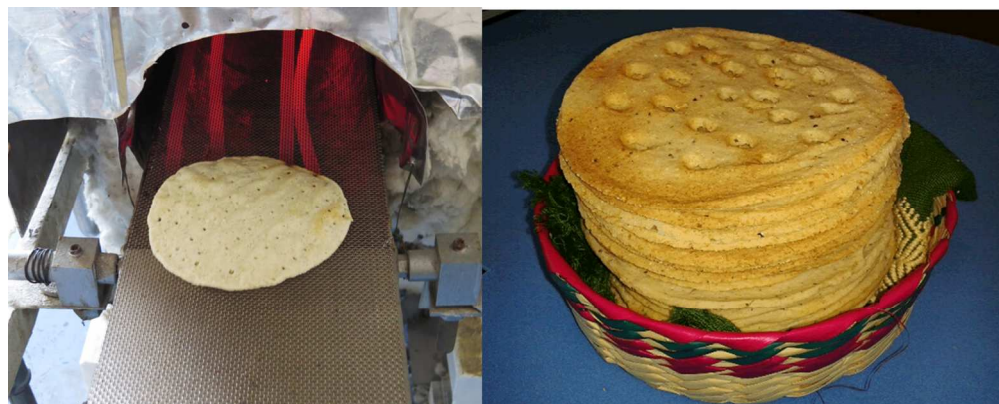
Figure 3. Infrared oven US Patent 5,567,457 (González-Henández et al 1996), used to elaborate the totopos (right side). Totopos with little holes made with either a finger or a comb, which prevents the fresh masa from ballooning up as they bake.
