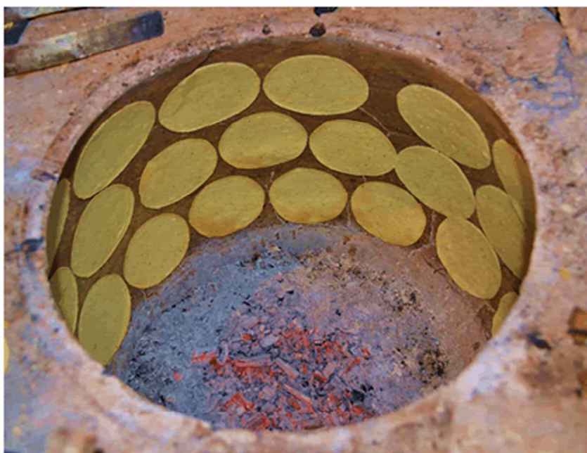
Figure 1. A cay hot oven (Comixcal or Comizcal) for preparing totopos by IR radiation. 169x127mm (72 x 72 DPI)
